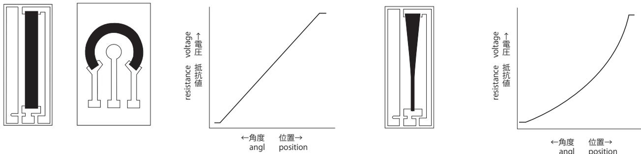
●屈折曲線特性 Refractive curve characteristics
